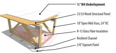
M4 Underlayment: Lightweight, No Curing Time, Installs Quickly with Glue / Nails / Staples, Mold / Pest / Abuse Resistant, Sealed, Noncombustible, No Silica, No Chloride & More
