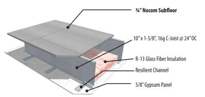
NOCOM Subfloor: No Curing Time, Installs Quickly with Screws, Sealed, T&G Edges, Mold / Pest / Abuse Resistant, Noncombustible, No Silica, No Chloride & More
